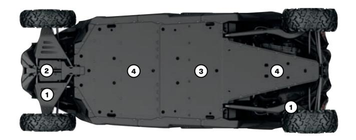
Our plastic plates glide smoothly and silently over obstacles, offering great protection in rough terrain. Made of abrasion-resistant thermoformed %" (10 mm) thick High Molecular Weight Polyethylene (HMWPE).
